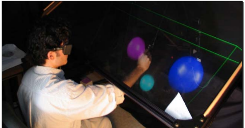
PARIS (Electronics Visualization Labs at The U. Illinois at Chicago) is a large-workspace, three-dimensional system that allows the user to see their own limb as well as virtual objects in space before them. This individual is holding the Phantom Robot (SensAble Technologies, Inc.) that renders programmed forces such as touching these artificial spheres.
