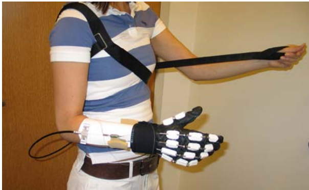
Fig. 1: Revised prototype for the HandAid. Redesign makes home use more feasible.
