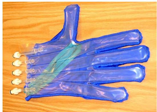
Fig. 2: Revised prototype of glove for PneuHand. Each digit has a separate air chamber for assistance.
