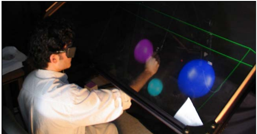
Demonstration using interaction with artificial spheres. VRROOM is a large-workspace, three-dimensional system that incorporates PARIS display (developed at EVL at UIC) that allows the user to see their own limb as well as virtual objects; a Robot that renders programmed forces, and a Flock of Birds motion tracking system.
