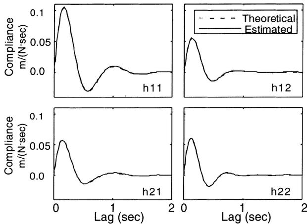
**Fig. 5.** Comparison of the estimated dynamic compliance impulse response functions (IRFs) (—) and those predicted from the known joint stiffnesses (---). Simulation data were obtained using the nonlinear model specified by (13).  $h_{ji}$  represents the SISO subsystem between input  $x_i$  and output  $y_j$
