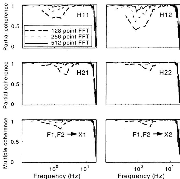
**Fig. 9.** Estimated partial and multiple coherence functions using FFT window sizes of 128 points (2.56 s; ---), 256 points (5.12 s; -.-), and 512 points (10.24 s; —)
