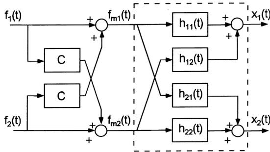
**Fig. 7.** Schematic of the model used to simulate a system with coupled inputs
