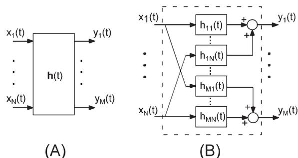
**Fig. 1.** **A** Block diagram of the structure used to represent a linear multiple-input, multiple-output (MIMO) system with inputs  $x_i$  and outputs  $y_j$ . **B** Equivalent subsystem representation
