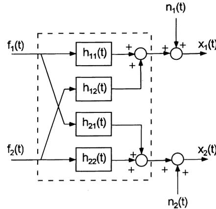
**Fig. 8.** Schematic of the model used to simulate a system with output measurement noise
