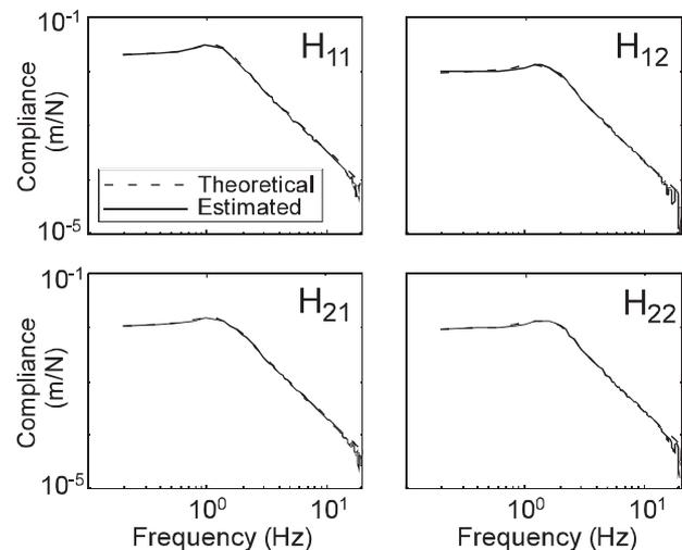
Fig. 3. Comparison of the estimated dynamic endpoint compliance transfer functions (TFs) (—) and those predicted from the known joint stiffnesses (---). Simulation data were obtained using the nonlinear model specified by (13).  $H_{ji}$  represents the single-input, single-output (SISO) subsystem between input  $x_i$  and output  $y_j$
