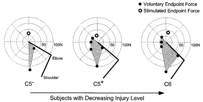
Fig. 5. Maximum voluntary endpoint forces. Shows the maximum forces generated by each of the tested arms along the measurement directions. The solid circles indicate the maximum voluntary forces and the open circles show the forces generated by triceps stimulation. The thick solid lines denote arm orientation. Note that all results are referenced to a right arm configuration.
