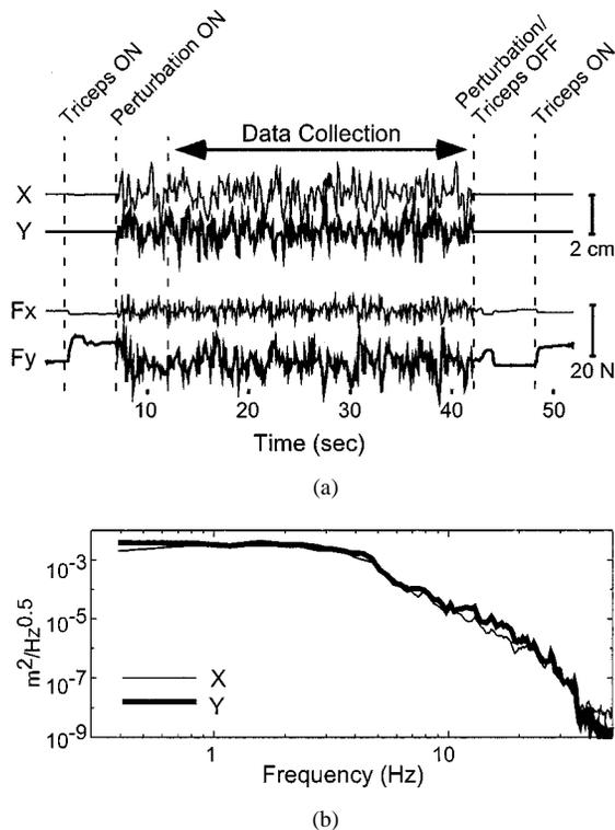
Fig. 3. Typical endpoint displacements and forces. (a) Typical displacements and forces during a single experimental trial. Dotted vertical lines indicate transition points in the experiment and are labeled above the figure. Only data between 12–42 s was used for subsequent analysis. (b) Power spectrum of the applied position perturbations.
