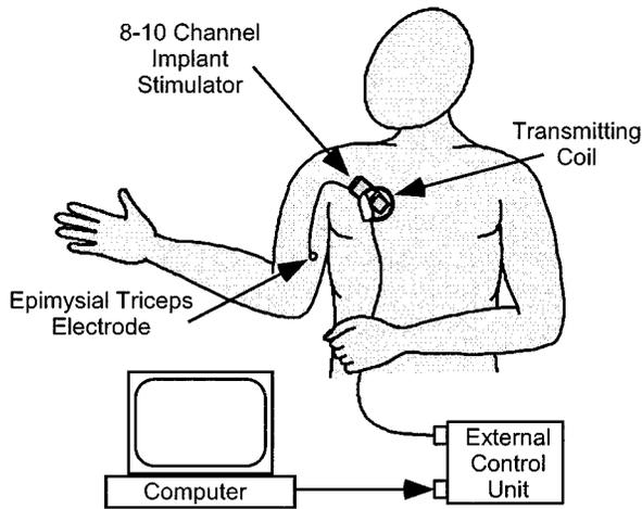
Fig. 1. Triceps FNS system. The portions of the implanted neuroprosthesis used for triceps stimulation are shown.
