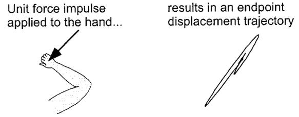
Fig. 4. Simulated transient responses. Illustrates the simulated endpoint trajectory in response to a unit impulse in endpoint force. The left portion shows the orientation of the force impulse and the right portion shows the corresponding endpoint trajectory (arbitrary scale). Arm parameters used during each such simulation were estimated from experimental data.
