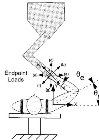
Fig. 2. Manipulator. A two-joint robotic manipulator was used to apply endpoint perturbations in these experiments. The manipulator was mounted on an adjustable structure, allowing its height to be customized for each subject. During each trial, subjects exerted a constant force on the manipulator in one of the eight directions shown.
