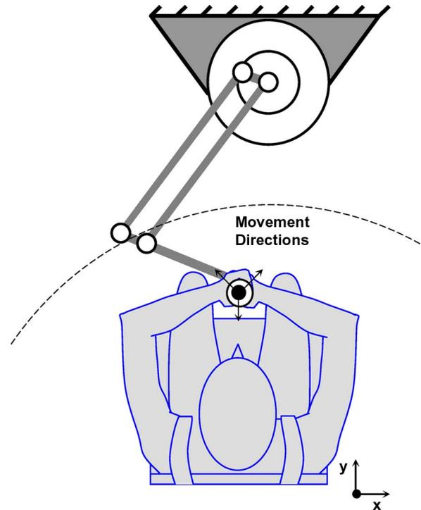
Fig. 1. Subject is seated at the planar manipulandum grasping the handle with a bimanual grasp. Forces are presented at the handle of the robot.
