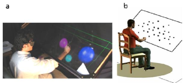
Fig. 1. The VRROOM system. (a) User seated at the apparatus with virtual spheres rendered both haptically and graphically. (b) An illustration of an experimental subject sitting in front of the VRROOM system, and the spatial arrangement of all possible virtual targets appearing within the 3D virtual environment.
