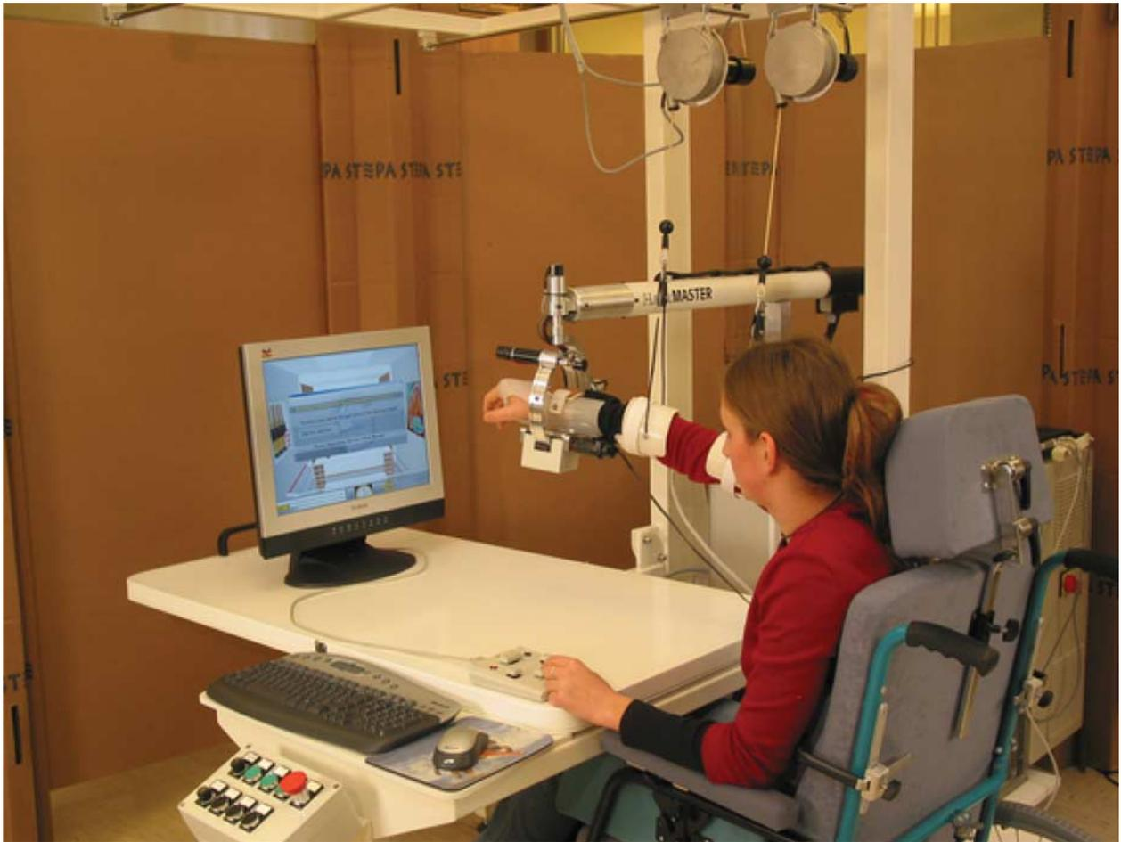
**Fig. 2.** Gentle/s commercial prototype for machine mediated neurorehabilitation.
