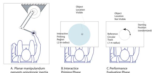
Fig. 1. (A) We simulated various anisotropic inertial loads with a force-feedback planar manipulandum. (B) Subjects were allowed to freely interact with each load in an "interactive priming" phase priming. (C) Following priming, subjects made circular movements with the manipulandum during an evaluation phase.
