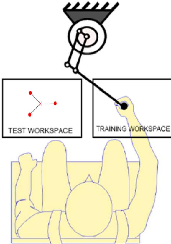
**Figure 1:** Subject seated in the chair in front of the manipulandum grasping the handle of the manipulandum. The arrangement of the workspaces and the targets are shown. (Figure not drawn to scale)
