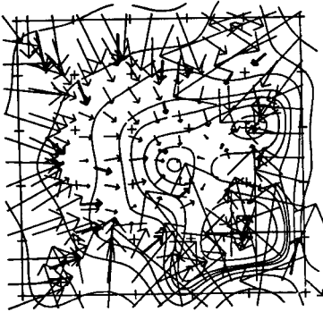
Fig. 6. Approximation of the samples shown in Fig. 5 ( bottom ) by a combination of 36 irrotational basis fields
